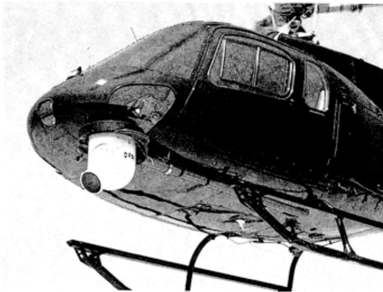
Figure 1 Left Front View of Installed mount with FLIR.
