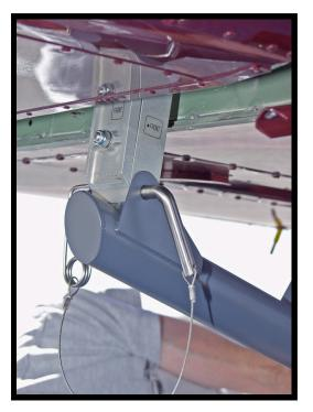
Attach both fore-to-aft Support Tubes to both front Skid Gear Clamps and secure with 7/16" Pins and safety-clips.
