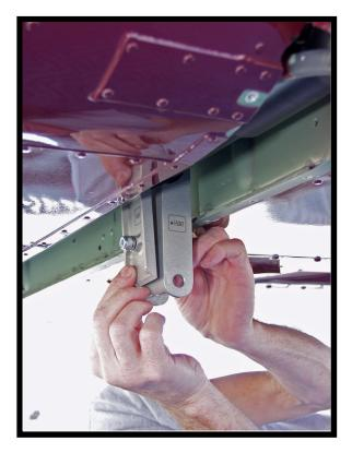
Install both Front and both Rear skid gear clamps. Note: Leave bolts loose so clamps can be shifted into position when attaching the Lateral Support Tubes. IMPORTANT: After all support tubes are attached, tighten all bolts and nuts.
