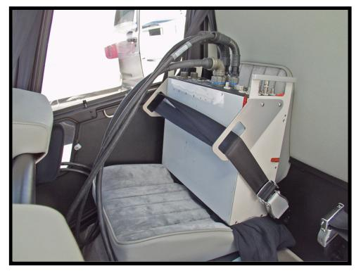
Fasten the FSI Camera Body Unit to a rear seat cushion with a seat belt. (Typically on the same side of the Video Gimbal)
