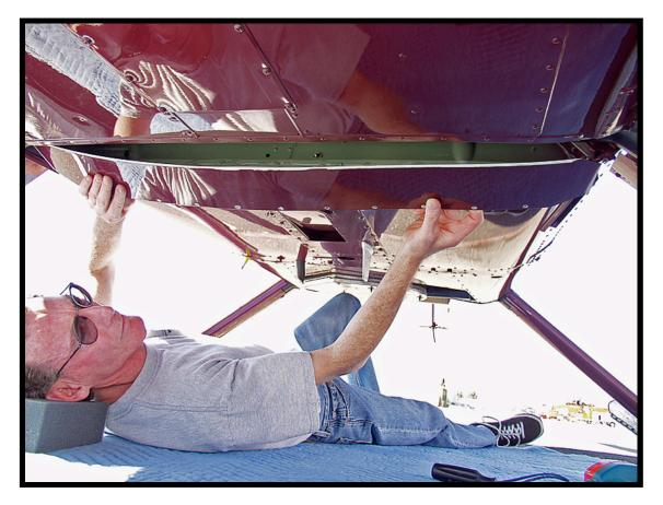
At the forward skid gear remove the forward skid gear cover.
