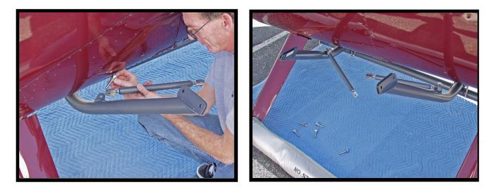
Install the two (2) diagonal tie-rods to the Lateral Support Tubes and secure with 3/8" PIP-pins.
