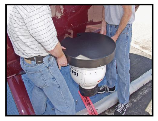
Attach the Video Gimbal (with suspension) to the vertical channels at the ends of the Lateral Support Tubes and secure with four (4) 3/8" PIP-pins.
