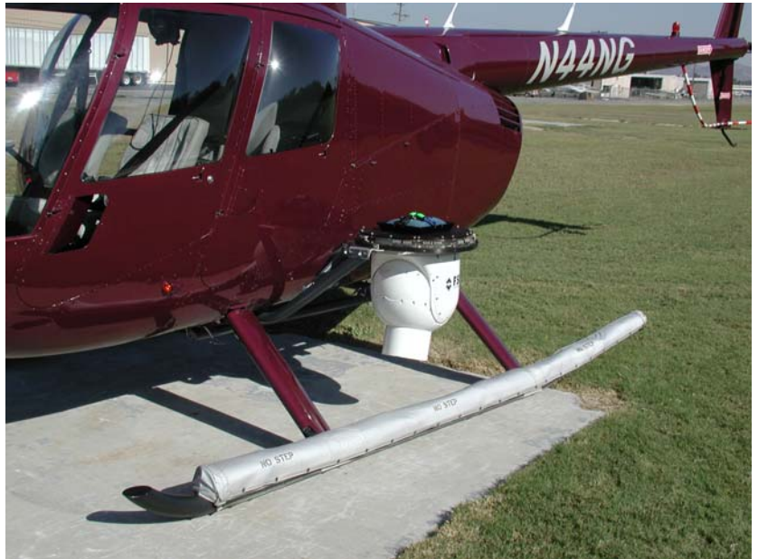
Figure 1. Camera Mount with a FLIR Ultra Media II (Typical Camera Installation)
