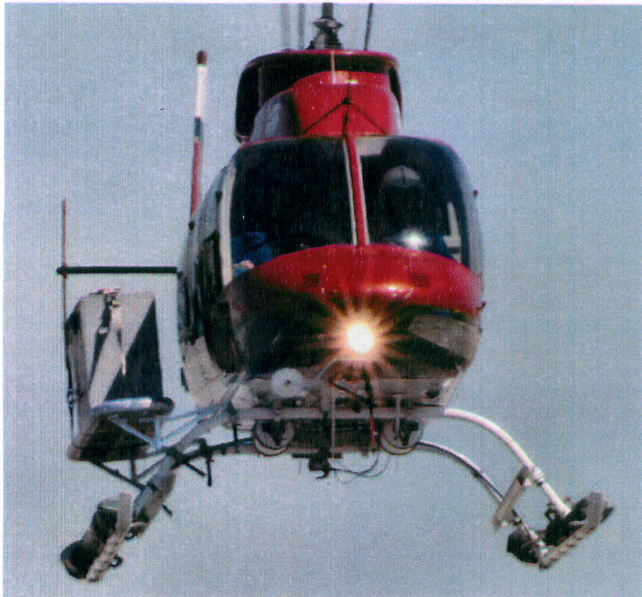
Figure 3 Front View of Right Rack with Load
