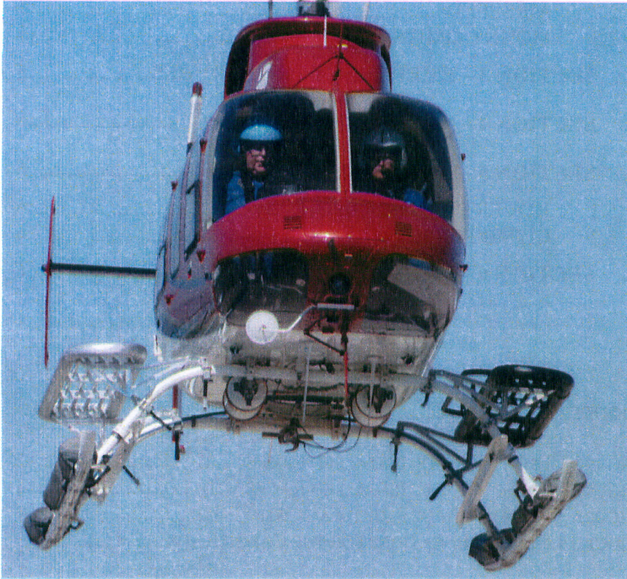
Figure 1 Front View of Installed Racks
