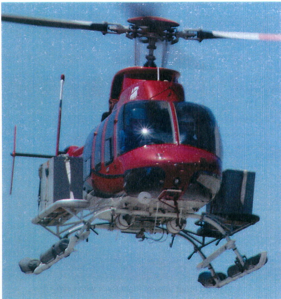
Figure 2 Front View of Installed Racks with Load
